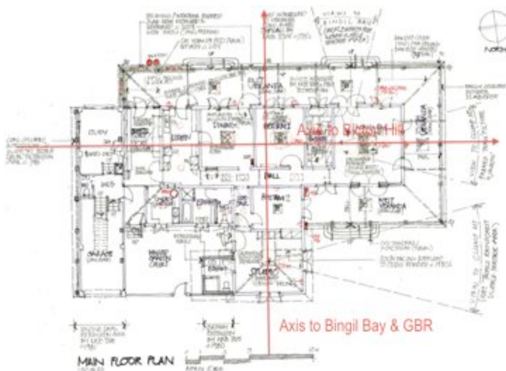
Fig 56. Main floor plan of Büsst's house annotated to show its primary orientation and layout (sketch plan from MGA site survey, Aug 2015)
