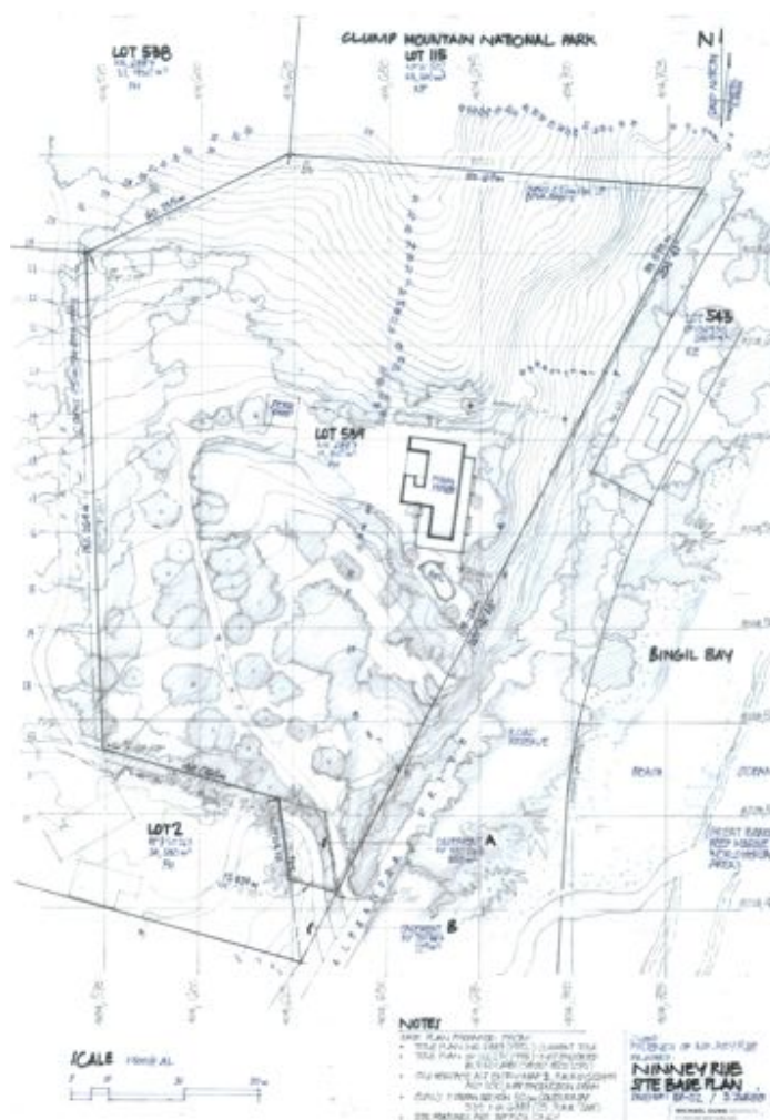
Fig 5. Top – QPWS aerial contour map 50cm (2015); Fig 6. Bottom – MGA Site Base Plan (2015) prepared as trace overlay from aerial contour with boundary data from title plan surveys.
